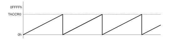
The TACCR0 CCIFG interrupt flag is set when the timer *counts* to the TACCR0 value. The TAIFG interrupt flag is set when the timer *counts* from TACCR0 to zero. Figure 11–3 shows the flag set cycle.
